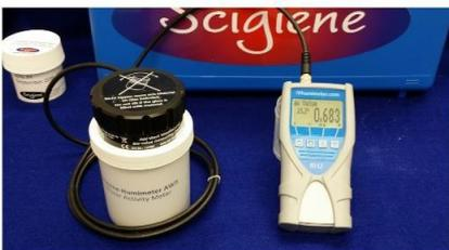
**Step 4: Turn on to Log Readings To Stability; typically < 5 minutes**
