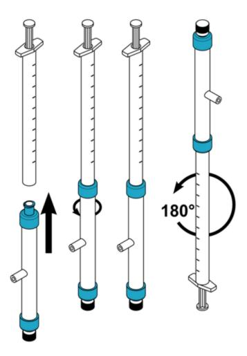
Keeping the filter upright, attach the 1ml syringe to the open end of the filter. Flip the filter and 1ml syringe 180°.
