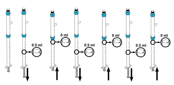
Pull the syringe back to the 0.5ml mark. Push the liquid all the way back into the filter. Repeat this step 2 more times.
