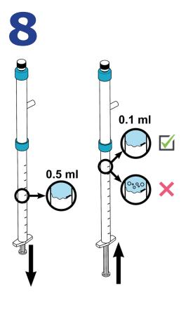
Pull the syringe back to the 0.5ml mark. Push the plunger in slowly to the 0.1ml mark to collect 0.1ml of sample exactly.
