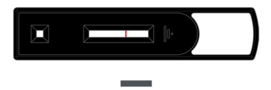
If no test line is present at the test line position but there is a control line, then the test is negative and Legionella pneumophila serogroup 1 has not been detected.
