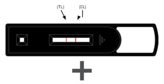
The test is composed of two lines; a test line (TL) and a control line (CL). If both lines are present, even if the test line is very faint, then Legionella pneumophila serogroup 1 has been detected above the cut-off of the test kit (>100 CFU/L).
