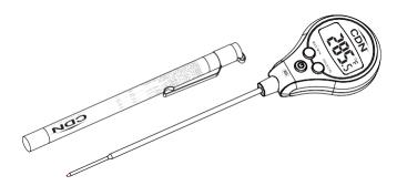
**Note:** Remove label from display before initial use. Clean the thermometer stem before each use.
