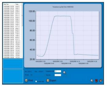
Software programs that automatically analyse data from sterilisation and pasteurisation
