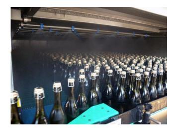
Ideally the process involves measuring internal bottle/can temperature relative to the external temperature of the spray and many processes involve recording internal product temperatures as well. (<u>SterilDisk</u> and <u>PasteurDisk</u>) dataloggers inside a dummy can/bottle or an outside probe (SterilCyl, PasteurCyl) inserted through special fittings to record internal temperatures are ideal here.
