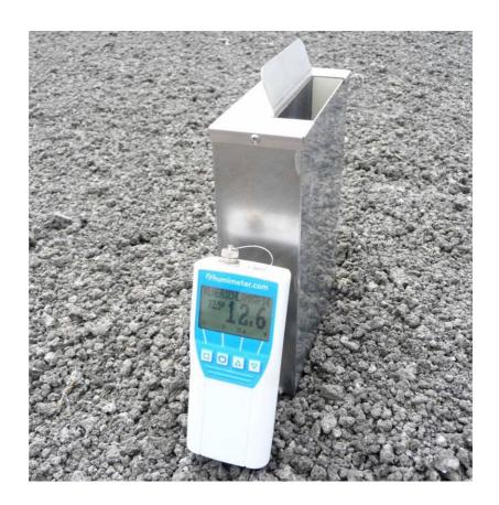
Sludge granulate moisture meter
