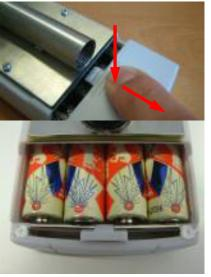
If the battery symbol appears in the measuring window resp. if a critical charge of battery is shown in the status, the batteries have to be changed IMMEDIATELY. If you do not use your humimeter device for a longer period, remove the batteries. For eventual resulting damages we cannot provide any warranty.
