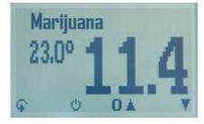
4.1. Marijuana cone (loose bud) sensor: To ensure correct measuring results, the measuring chamber has to be full to the brim with material, but must not be precompressed (see illustration picture). Put the cap (compressing fixture) onto the measuring chamber and tighten it to the stop. As soon as the measuring chamber is completely closed, the display shows the measuring value.
