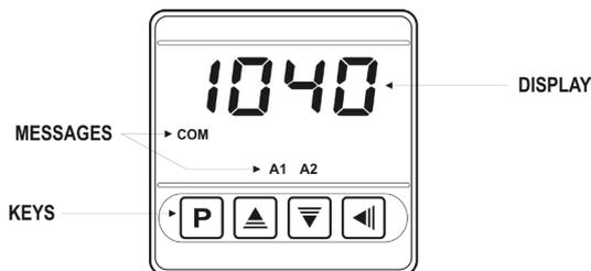
Figure 06 - Identification of the front panel parts
