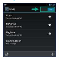
Turn on Wi-Fi if it is off. Select the wireless network to connect to. If you cannot find the wireless network to connect to in the list touch the Add (+) icon to manually add it.
