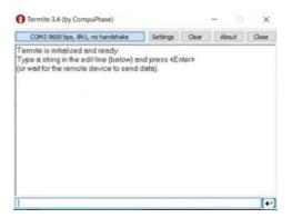
2. On the Terminal Software select the Computer COM port where the Spin Air is connected and set the following communication parameters:
