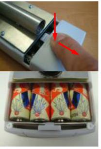
If the battery symbol appears in the measuring window resp. if a critical charge of battery is shown in the status, the batteries have to be changed IMMEDIATELY. If you do not use your humimeter device for a longer period, remove the batteries. For eventual resulting damages we cannot provide any warranty.
