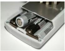
If the battery symbol appears in the measuring window resp. if a critical charge of battery is shown in the status, the batteries have to be changed IMMEDIATELY.
