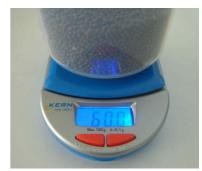
7. Fill up the measuring device with the sample material. The filling needs to be done <u>slowly and constantly</u> to ensure reproducible results. There must not be used a funnel or anything similar for filling.
