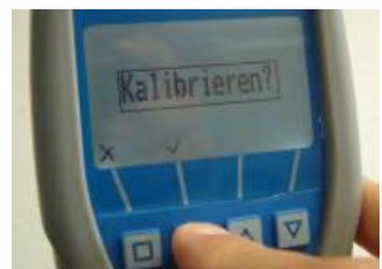
Hold the humimeter GF2 in one hand up in the air and make sure that nothing stands behind the black measuring plate. Now press the second button (**✓**) with one finger.
