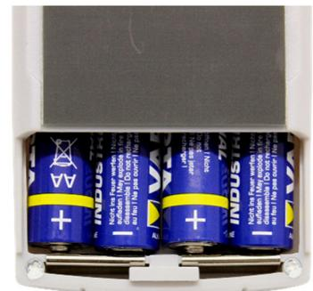
If the battery symbol appears in the measuring window resp. if a critical charge of battery is shown in the status (!), the batteries have to be changed IMMEDIATELY. If you do not use your humimeter device for a longer period, remove the batteries. For eventual resulting damages we cannot provide any warranty.
