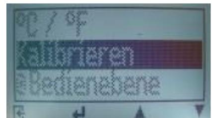
This menu item has to be unlocked. For that you have to enter the 4-digit serial number of your humimeter. You can find the serial number on the top right edge of the display a short time after switching on the instrument, or on the sticker in the battery slot.
