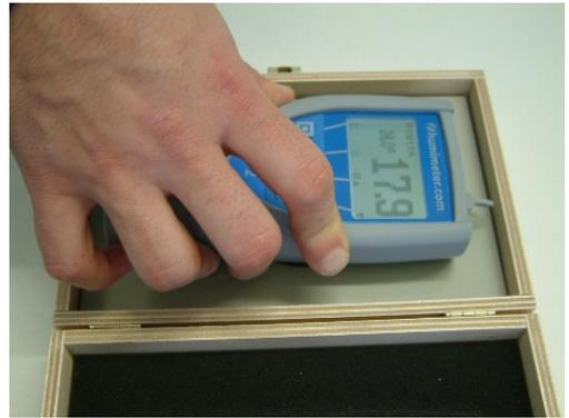
The shown measuring value should range between **17.5** and **18.5**. If the shown value is out of this range, you have to carry out a calibration (see instructions below).
